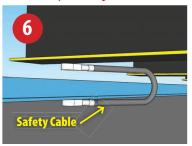
**Step 6—Install Safety Cables**Secure Safety Cables to aluminum angle on back of panel and crossmember flange using supplied Tek Screws or optional 1/4-inch bolts. **Cable must be looped to allow enough slack for a full range of movement.**
