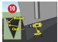
**Step 10—Install Rubber**Drill the rubber using the holes at the bottom of the panels for guides. Fasten with long aluminum rivets and a square aluminum washers. **The rubber skirt has a cleat that aligns with the bottom of the panel.**
