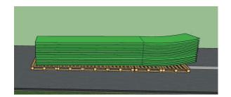
**Aluminum Crossmembers Require Shims!** The shims are placed underneath the clamps.
