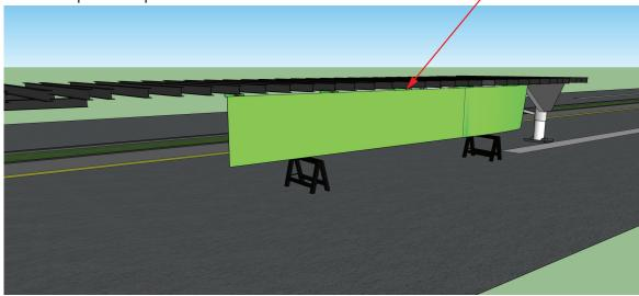
Install the Turn Signal Light. Install the turn signal light according to legal requirements. The panel can be cut with a hole saw or a jig saw.
