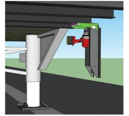
An impact wrench works best. The torque spec is 20 ft. lbs.
