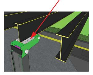
If installing on *steel* crossmbers, *discard* the shims.
