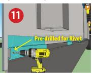
**Step 11—Install and Secure Rubber Skirt** The first and last clips are pre-drilled for rivets. Drill through the rubber and panels, then fasten the rubber with a rivet. **Only secure the rubber to the first and last clips**.
