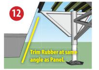
**Step 12—Trim Rubber Skirt** On the leading edges of the skirt, match the angle of the front panels and trim the skirts.
