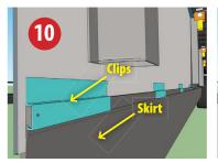
**Step 10—Install Rubber Skirt** The rubber skirt slides into the aluminum clips that are mounted to the backs of the panels.
