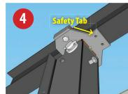
Step 4—Secure Safety Tab with Screw Use the provided Tek Screw to secure safety tab. Secure one side only.
