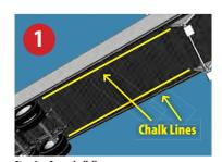
Step 1—Snap chalk lines. Refer to the Layout Guide for the appropriate Aerodynamic Configuration Number (AC#). IMPORTANT: Illustration above is a representative sample only. There are numerous aerodynamic configurations.
