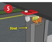
Step 5—Install Remaining Struts Install remaining Struts before hanging panels. Refer to layout on the reverse side for Strut placement.
